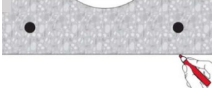
3. Marking pre-stressed steel position
