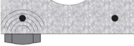
1. Positioning pre-stressed steel
