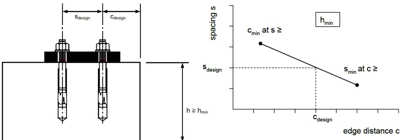
**FIGURE 2 – INTERPOLATION OF MINIMUM EDGE AND SPACING DISTANCE**
